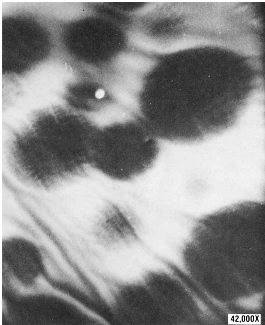
Fig. 10. Transmission electron microscope scan of the epoxy blend/copolyester system described in Figure 9, prior to heating.
